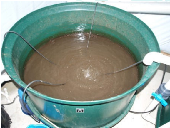
Figure 5: Separated, aquatic, media-less fish waste solids mineralisation tank. NZ, semi-commercial, NFT aquaponic system.
